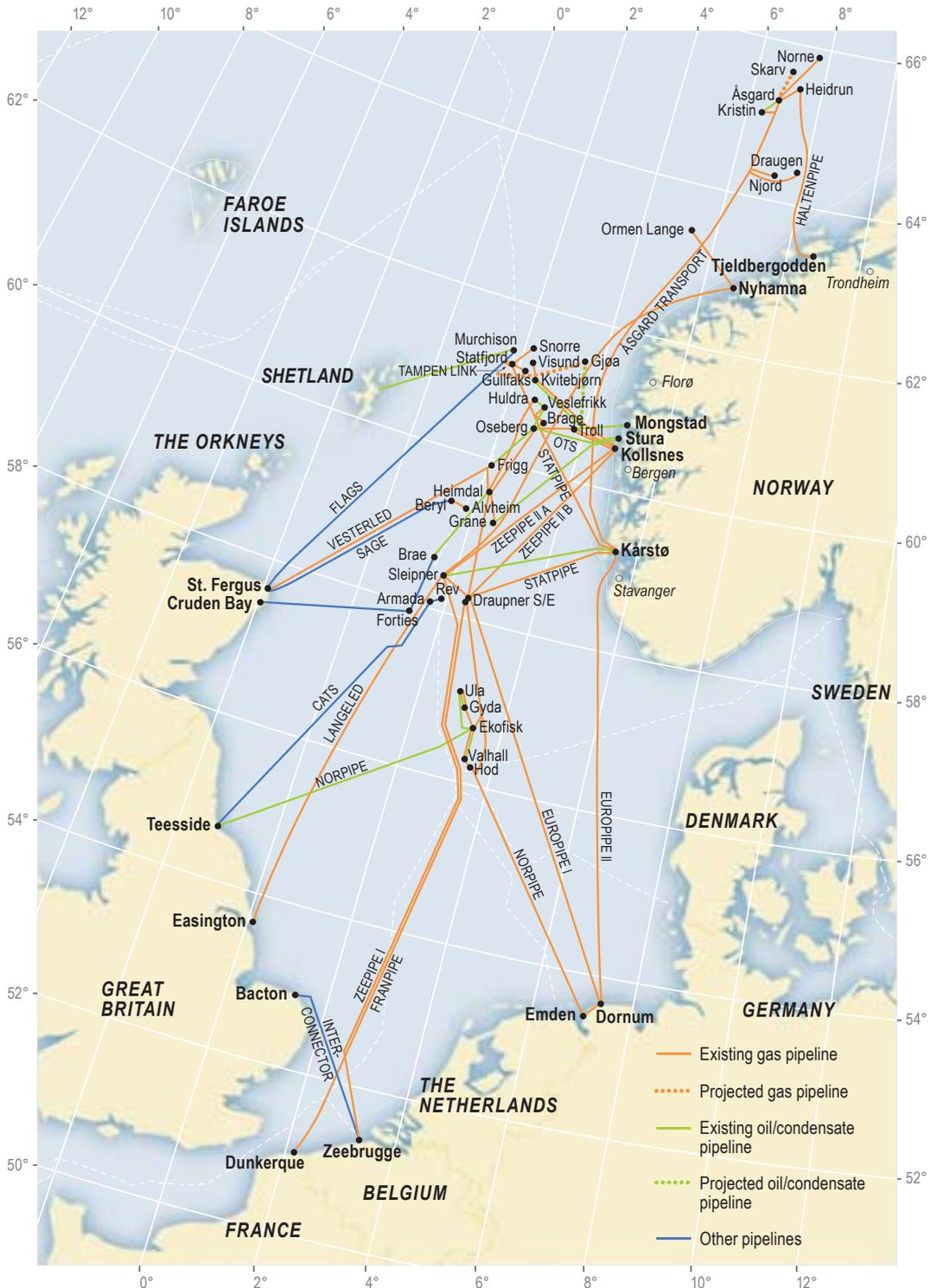
**Figure 15.1** Existing and projected pipelines
