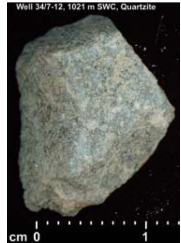
Fig 5: Sharp-edged quartzite stone found in a sidewall core close to the base of the unit interpreted by Statoil as the Utsira formation. This piece of rock hails from the mainland and must have been carried to the Tordis area during the ice age – long after the Utsira was deposited.
