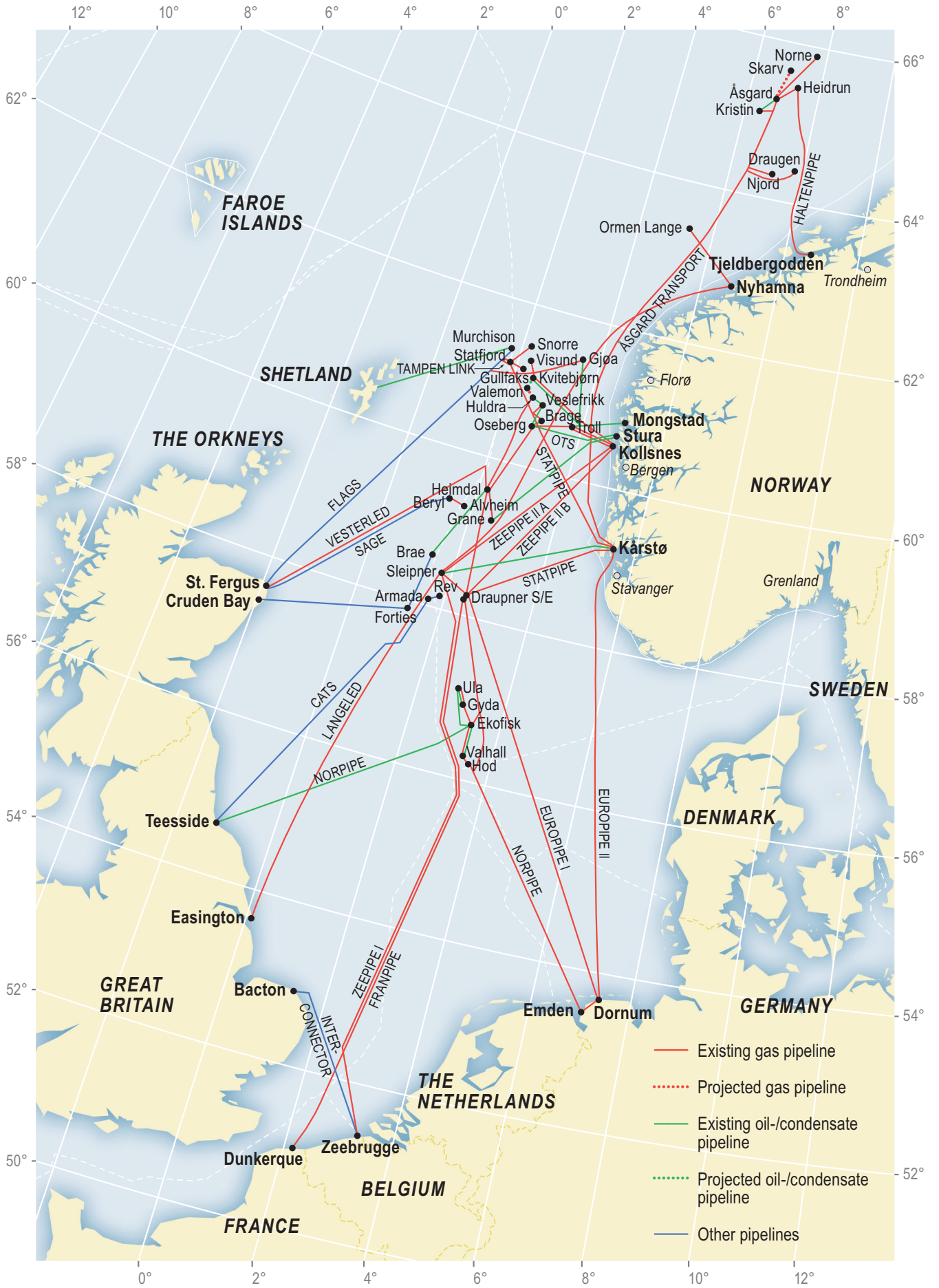
Existing and projected pipelines (Source: Norwegian Petroleum Directorate)
