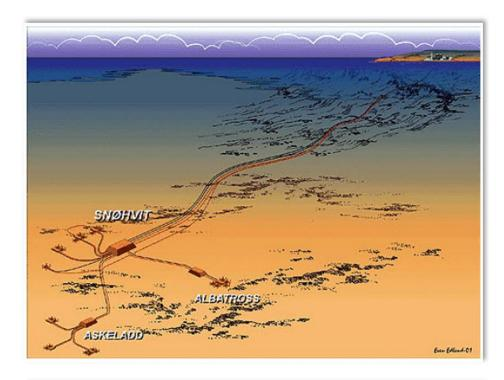
The <u>Snøhvit</u> gas field in the Barents Sea. The well stream, with natural gas, CO<sub>2</sub>, NGL and condensate, is transported in a 160-kilometre pipeline to the facility onshore. The gas is processed and cooled down to liquid natural gas (LNG). The CO<sub>2</sub> is separated and returned to the field by pipeline for reinjection into a formation in the same field.
