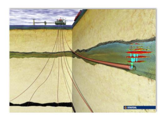
The <u>Sleipner</u> gas field in the North Sea. This is the world first offshore CCS project. Today, three hydrocarbon fields capture  $CO_2$  through the <u>SleipnerT</u> facility and inject through the same well in the aquifer in <u>Utsira</u> formation.
