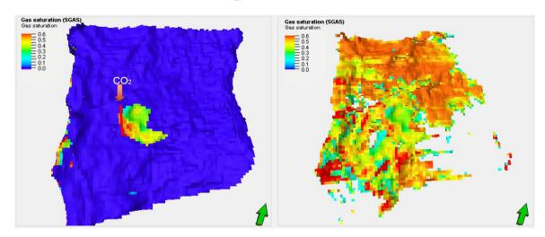
Fig. 3 CO<sub>2</sub>/gass saturation is observed from the top of the reservoir (in the left) and the distribution of the gas in all layer of the reservoir (right) after stop injection of the case with 6.2% increase of oil recovery, 12 Mt CO2 injected in one existing-injection well and 87% of the gas is stored in the reservoir.
