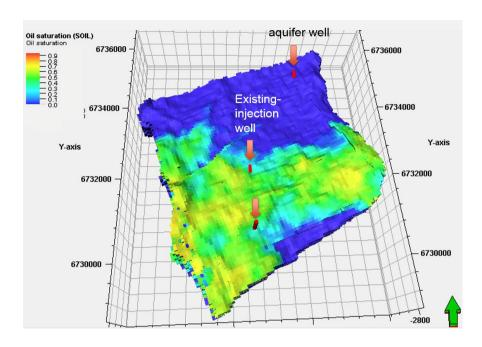
Fig. 2: reservoir model with different location of CO<sub>2</sub> well injection.
