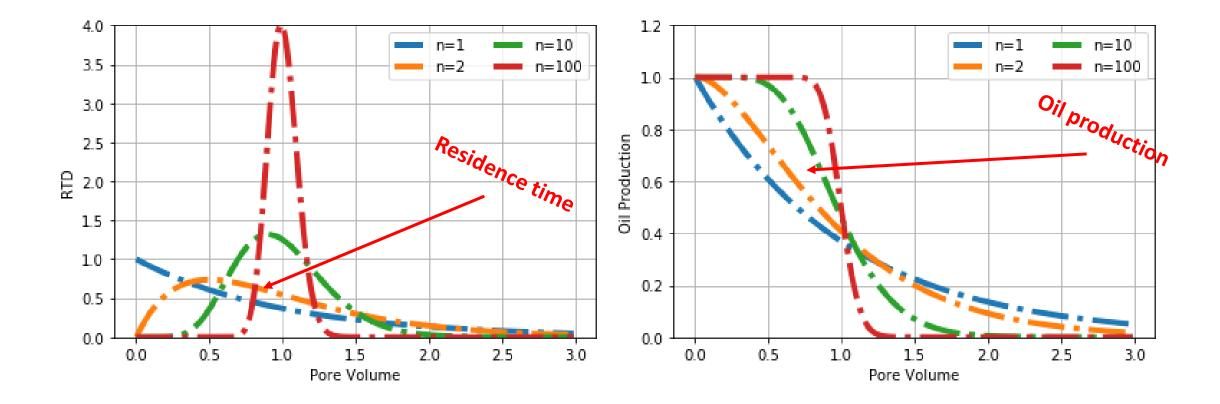
"n" represents a heterogeneity factor  $n \rightarrow \infty \Rightarrow$  piston displacement (homogeneous)
