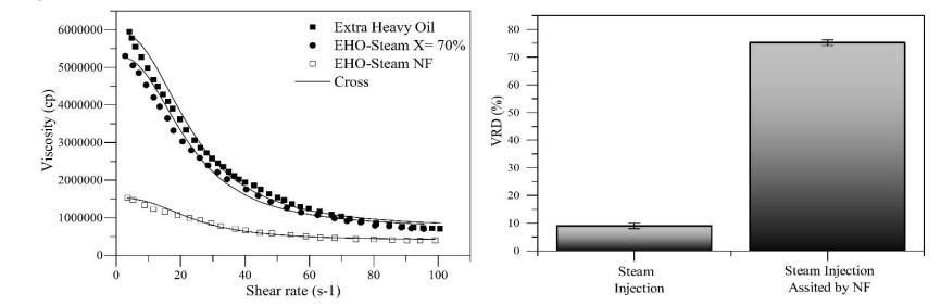
**Figure 7.** (a) Oil recovery curve for steam injection assisted by CeNi0.89Pd1.1 nanocatalyst. (b) Rheological behavior and (c) viscosity reduction of oil recovered in each stage
