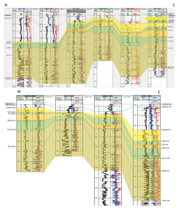
Well section panels showing gamma and neutron/density logs reflecting thickness variations of the different formations. The Åre and Tilje Fms show more or less constant thickness throughout the area. The lle and Garn Fms are thinning and shaling out towards the north. The Garn Fm is quite thick in well 6510/2-1, but less sandy, and is thinning towards the west.
