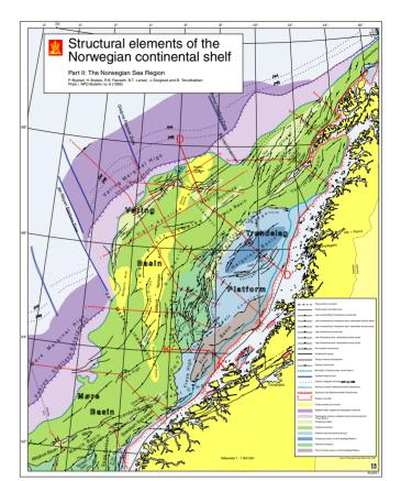
Structural element map of the Norwegian Sea. The Trøndelag Platform is shown by blue and gray colours. The depth and thickness maps in the following pages cover the Trøndelag Platform.
