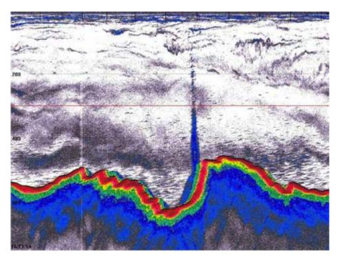
Detection of gas bubbles by echo sounder systems. The figure shows the acoustic signature generated by CO<sub>2</sub> bubbles being naturally released from the Jan Mayen vent fields. The CO<sub>2</sub> bubbles are here seen as a blue flare that rises around 500 metres from the seafloor through "clouds" of plankton in the water column.
