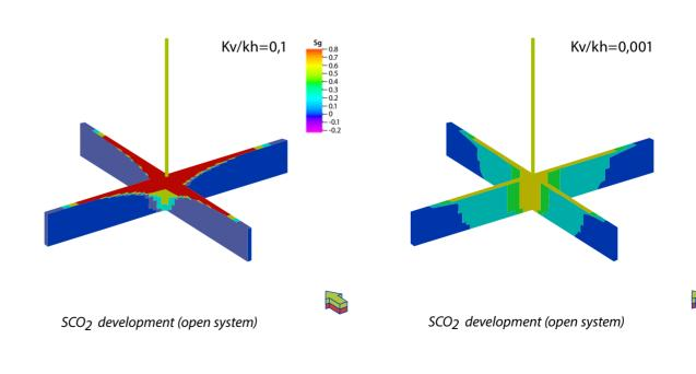
A cross section of a flat reservoir with injection for 50 years.
