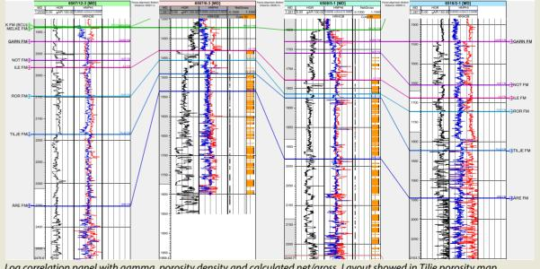
Log correlation panel with gamma, porosity density and calculated net/gross. Layout showed in Tilje porosity map.
