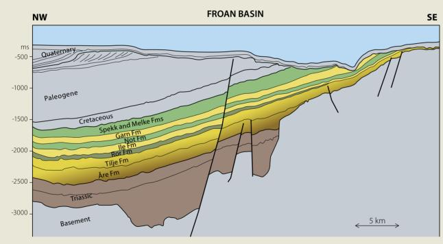
NW-SE profile showing the geometry of aquifers (yellow) and sealing formations (green) in the simulation model.
