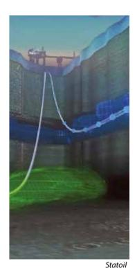
Sleipner: More than 13 million tonnes of carbon dioxide are now stored in the Utsira formation in the North Sea. Every year since 1996, one million tonnes of carbon dioxide has been captured from natural gas production at the Sleipner field, and stored in an aquifer more than 800 metres below the seabed. The layer contains porous sandstone filled with saline water.
