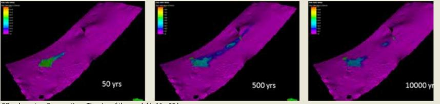
CO<sub>2</sub> plume top Garn vs. time. The size of the model is 16 x 35 km.
