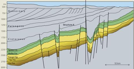
*NW* – *SE* profiles across the SE flank of the Helgeland Basin. The closed structures A and B are indicated. The location is shown in p. 44.
