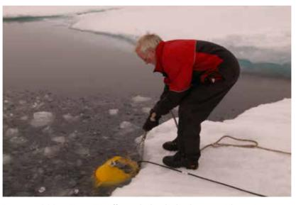
**Data acquisition.** Yngve Kristoffersen deploys hydrophones to pick up seismic signals. About 1 000 kilometres of such data were acquired during the expedition. (Photo: Audun Tholfsen)
