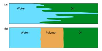
Figure 2.14 Polymer flooding.
