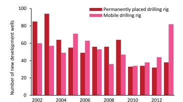
Choosing a development solution with permanent or mobile rigs depends on such considerations as the extent of the reservoir, its complexity and the water depth. Differences in drilling efficiency
