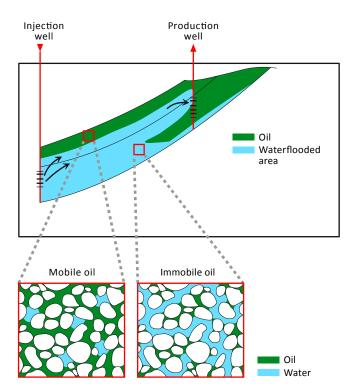
Figure 2.13 Cross-section of a reservoir showing an example of oil and water distribution after waterflooding, and distribution of the liquids at pore level. IOR methods can be categorised as conventional or advanced. The latter (less mature) methods are often termed enhanced oil recovery (EOR). They involve advanced flooding methods intended to help mobilise part of the immobile oil. See figure 2.13.
