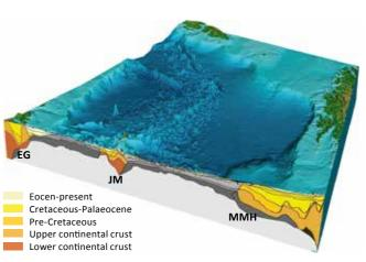
**Figure 7.7** A geological cross-section of the Norwegian Sea from eastern Greenland (EG) in the west, across the JMM, to Norway (MMH). The two major continents on either side of the sea are coloured in yellows and browns in the same way as the microcontinent. The grey strata between the continents comprise young seabed crust formed of volcanic rocks without petroleum potential (crustal cross-section taken from Mjelde et al, 2008, Marine Geophysical Researches).
