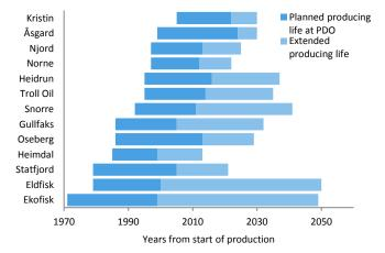
Figure 4.11 Planned producing life at the PDO date for fields with processing facilities, and extended producing life based on current plans
