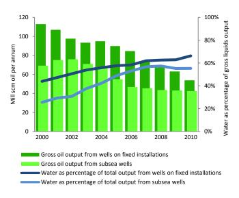
Figure 5.2 Distribution of oil production and water cut from subsea wells and wells on fixed installations, 2000-2010
