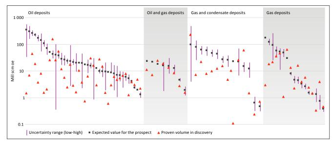
Figure 2.4 Comparison of operator expectations of petroleum volume in 67 deposits before drilling, and the results after drilling
