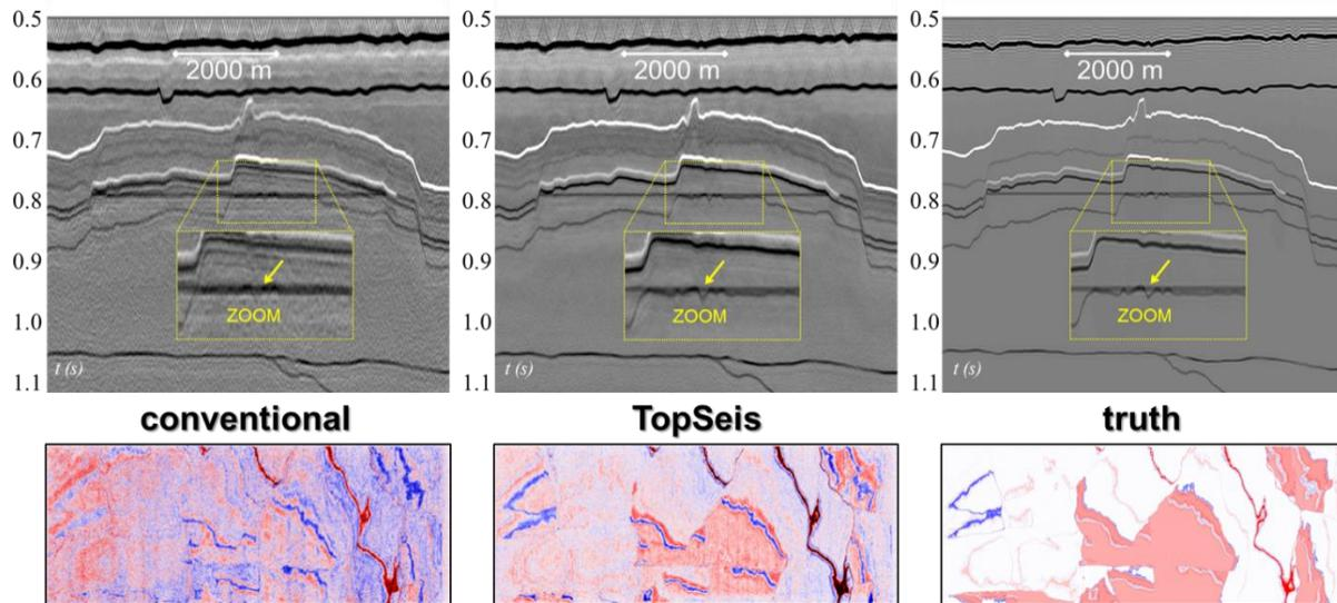
Figure 3: Migrated stacked images with zooms on the oil-water contact (top row) and extracted AVO gradient ( $G$ ) parameter along the oil water contact (bottom row) for a conventional marine survey (left column), a TopSeis solution (middle column) and the true reflectivity/AVO model (right column).
