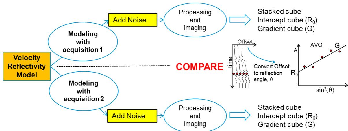
Figure 1: Schematic view of evaluation of seismic surveys based on modelling and processing/imaging
