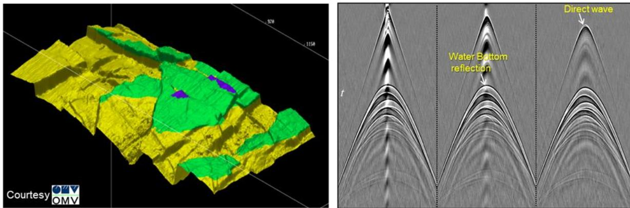
Figure 2: Example of diffraction modelling: Top Reservoir with reflectivity (left) and synthetic shot gather in three streamers with noise (right)
